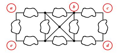
If  $V_{ab} = 10 \text{ V}$ ,  $V_{ac} = 5 \text{ V}$ ,  $V_{ae} = 1 \text{ V}$  and  $V_{db} = 3 \text{ V}$ :
